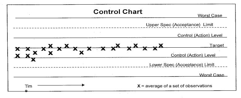
By monitoring the results of changes of inputs through control charting, the resultant variation in output can be determined and inherent variation of the process identified. Ultimately, control charting may be used to continuously monitor the process and assure a state of validated control. Control or action levels can be determined to adjust the process and maintain the process within the control limits.
