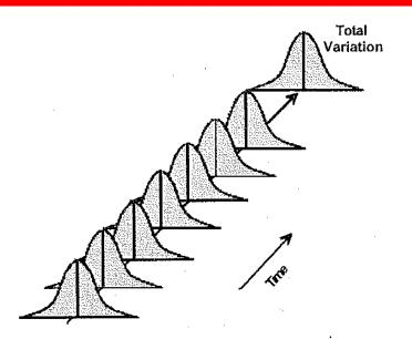
However, stability is not the only thing required. Once a consistent performance has been achieved, the remaining variation must be made to safely fit within the upper and lower specification limits. Such a process is then said to be stable and capable. Such a process can be relied on to consistently produce good product as illustrated in figure 6.
