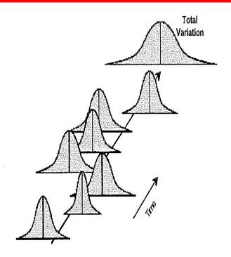
Instead, stable processes are desired as shown in figure 5. Stable processes produce a consistent level of performance. The total variation is reduced. The process is more predictable.
